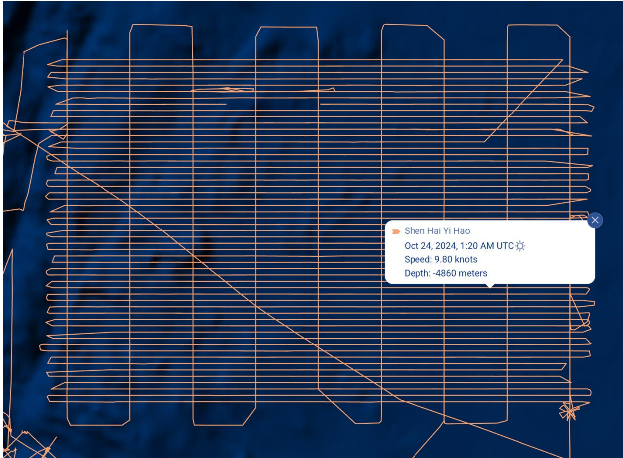
Figure 2: The lawnmower pattern of Shenhai 1 in the Philippine Sea. Vessels that are mapping typically travel at a speed of 8-10 knots. This AIS data can be retrieved from Global Fishing Watch.
